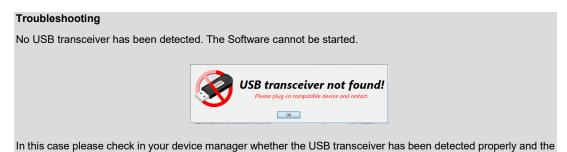
driver is installed. If the driver is missing, you may download the appropriate driver for your system from
