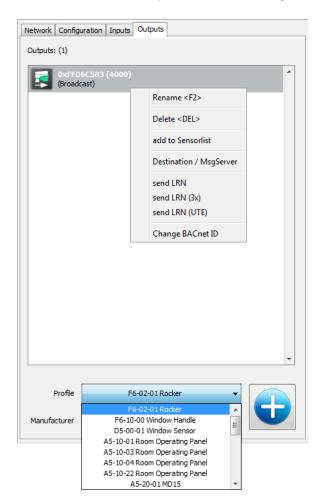
Click right on a particular sensor icon to open the context menu and select **<send LRN>** to send a Learn-in message to the device that is to be paired with this message.
