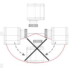
3. Note the mounting position. (Type of protection IP40)
