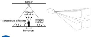
The sensor lense divides the detection area in 32 measurement areas. The sensor detects changes in infrared radiation that occur when an object\* (or person) moves that has a different IR temperature than its surroundings
