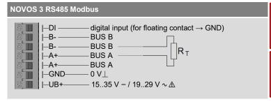
With alternating voltage, the correct polarity must be ensured!
