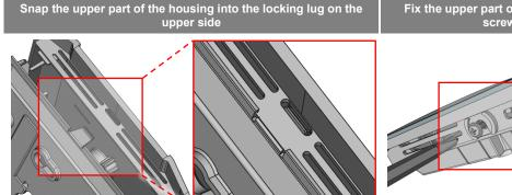
Fix the upper part of the housing on the underside with the screw included in the delivery.
